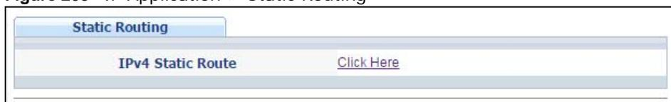
To enable IPv4 static route, configure the static route settings in the **IP Application > Static Routing > IPv4 Static Route** screen.
