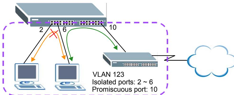
Note: Make sure you keep at least one port in the promiscuous port list for a VLAN with private VLAN enabled. Otherwise, this VLAN is blocked from the whole network.
