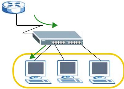
**Figure 87** Static Multicast Forwarding to Multiple Ports
