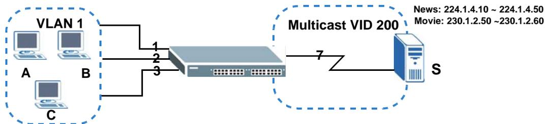
To configure the MVR settings on the Switch, create a multicast VLAN in the **MVR** screen and set the receiver and source ports.
