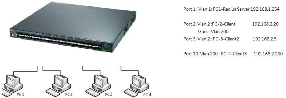
In this scenario, PC 2 will be authenticated. If the authentication succeeds, it will join VLAN 2 and should be able to communicate with PC 3. When it fails to authenticate, it will join guest VLAN and will only be able to communicate with PC 4.
