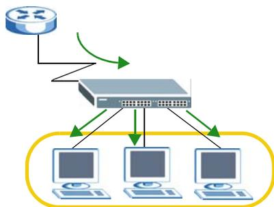
**Figure 83** Static Multicast Forwarding to A Single Port
