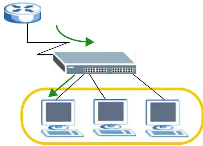
**Figure 84** Static Multicast Forwarding to Multiple Ports
