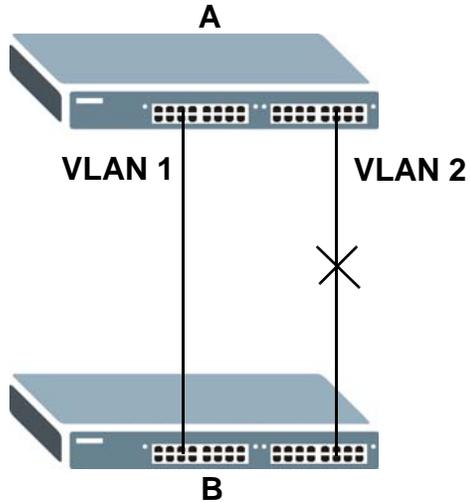
With MSTP, VLANs 1 and 2 are mapped to different spanning trees in the network. Thus traffic from the two VLANs travel on different paths. The following figure shows the network example using MSTP.
