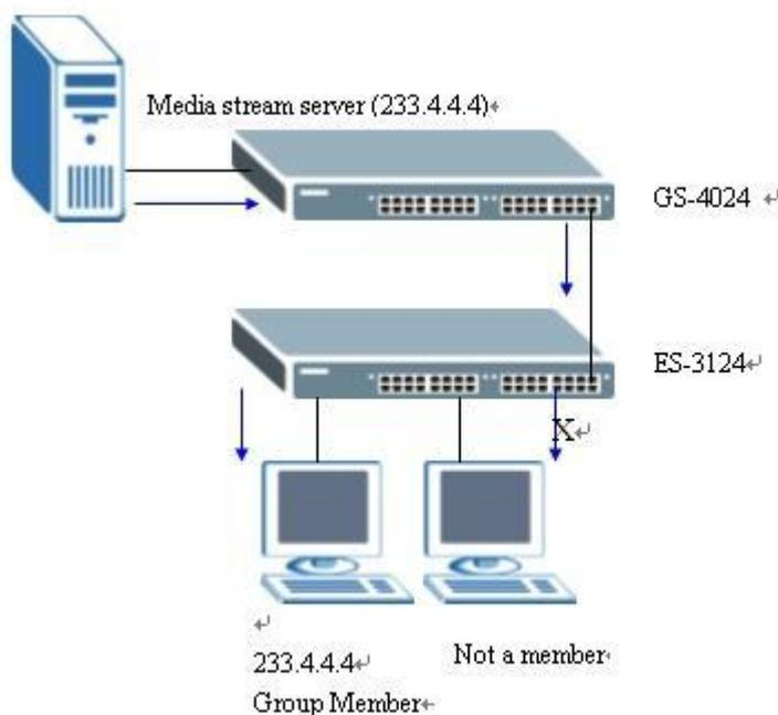
**Step one:** In the GS-4024 GUI, click the **IP Application IGMP**. Here, both versions of the the IGMP function can be enabled ( IGMP-v1 and IGMP-v2). At this case, we enabled IGMPv2 for both IP Domain.
