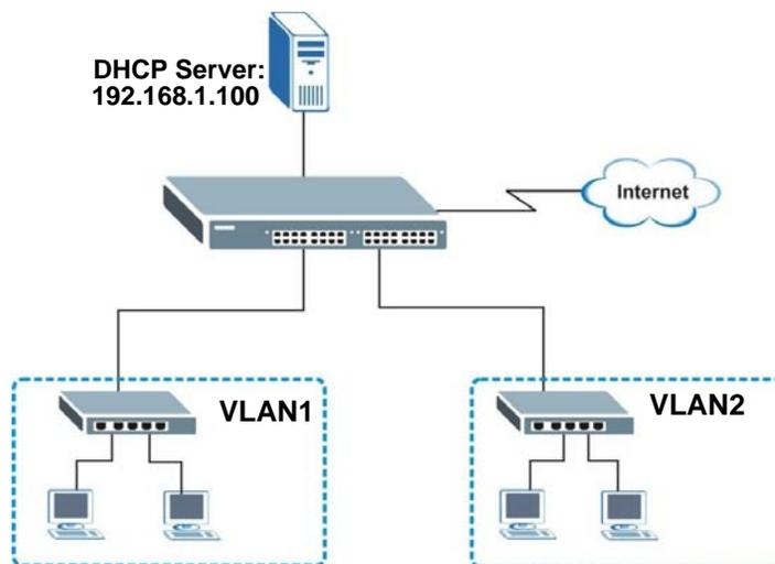
Configure the **DHCP Relay** screen as shown. Make sure you select a DHCP option 82 profile (**default1** in this example) to set the Switch to send additional information (such as the VLAN ID) together with the DHCP requests to the DHCP server. This allows the DHCP server to assign the appropriate IP address according to the VLAN ID.
