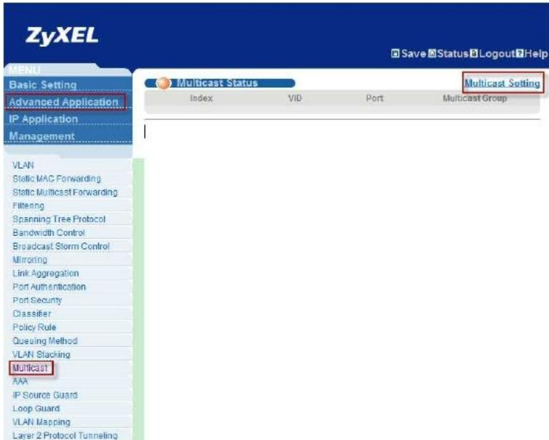
**Step three:** enable IGMP snooping function using the Web-GUI.
