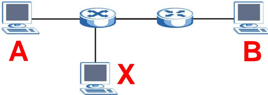
In this example, computer **B** tries to establish a connection with computer **A**. Computer **X** is in the same broadcast domain as computer **A** and intercepts the ARP request for computer **A**. Then, computer **X** does the following things:
