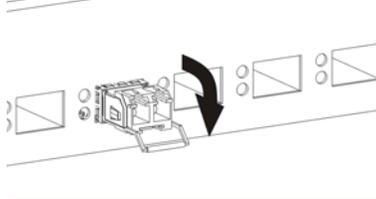
**Figure 15** Transceiver Removal Example
