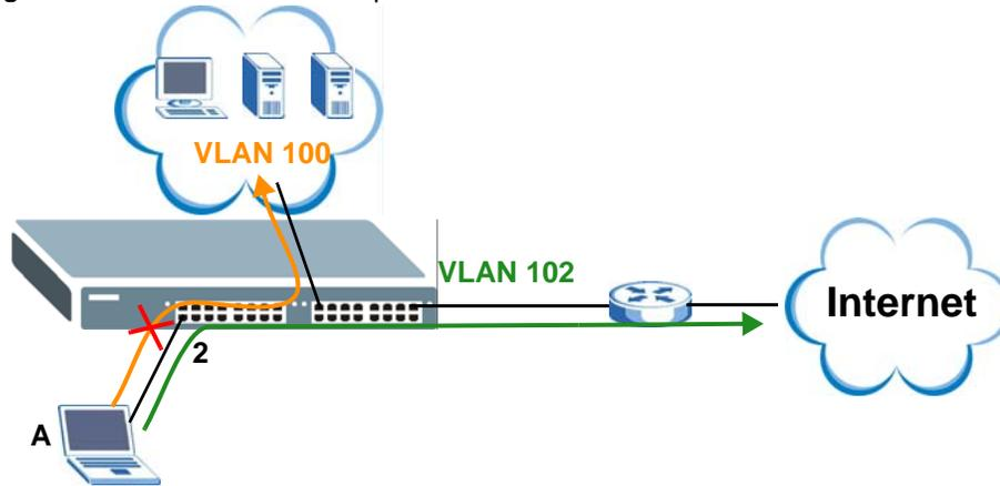
Use this screen to enable and assign a guest VLAN to a port. In the **Port Authentication > 802.1x** screen click **Guest Vlan** to display the configuration screen as shown.
