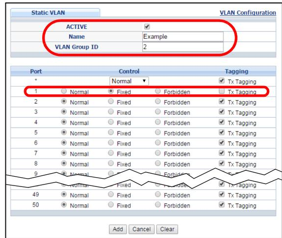
Note: The **VLAN Group ID** field in this screen and the **VID** field in the **IP Setup** screen refer to the same VLAN ID.
