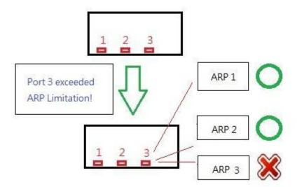
This is very useful when combined with Errdisable recovery, because the port put into ErrDisable can be recovered automatically in period of time. So it can protect switch's CPU without completely shutting down a network connection.
