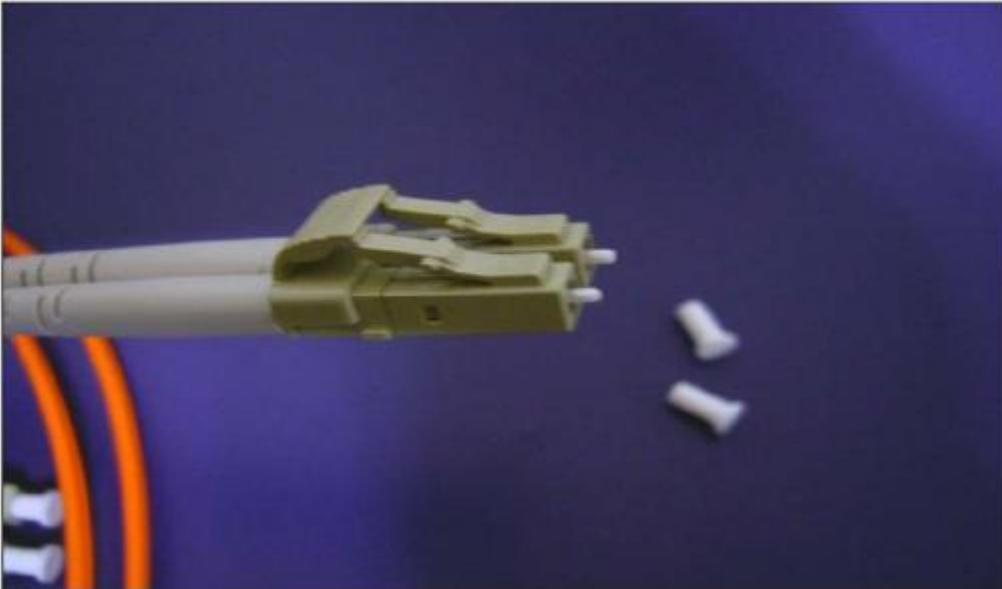
5. Plug the LC/LC Fiber Cable into the transceivers on both Switch.
