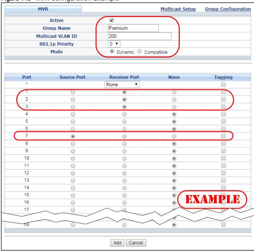
Figure 145 MVR Configuration Example
