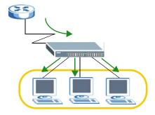
Figure 86 Static Multicast Forwarding to A Single Port
