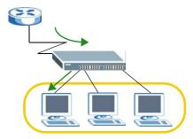
Figure 87 Static Multicast Forwarding to Multiple Ports
