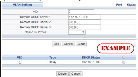
Figure 221 DHCP Relay for Two VLANs Configuration Example
