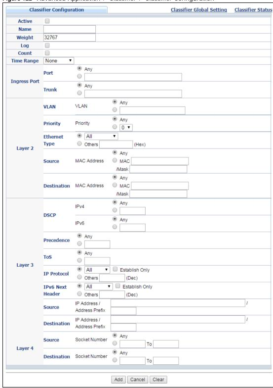
Figure 122 Advanced Application > Classifier > Classifier Configuration
