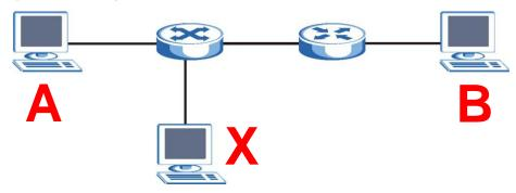
In this example, computer  ${\bf B}$  tries to establish a connection with computer  ${\bf A}$ . Computer  ${\bf X}$  is in the same broadcast domain as computer  ${\bf A}$  and intercepts the ARP request for computer  ${\bf A}$ . Then, computer  ${\bf X}$  does the following things:
