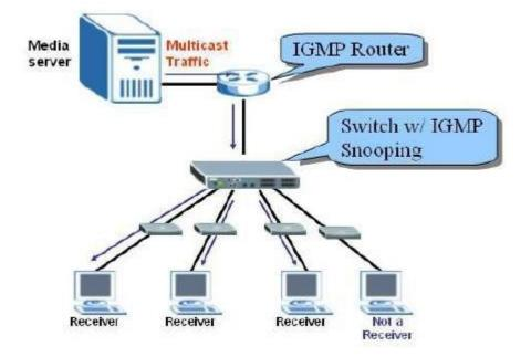
IGMP snooping is designed for application with deployment of multicast traffic. It operates on the underlying IGMP mechanism where a layer two switch passively listens to the IGMP Query, Report and Leave (IGMP version 2) packets transmitted between the IGMP router and clients, and collects passing IGMP messages. Also, the switch records the message's group registration information and configures multicasting information accordingly. If the
